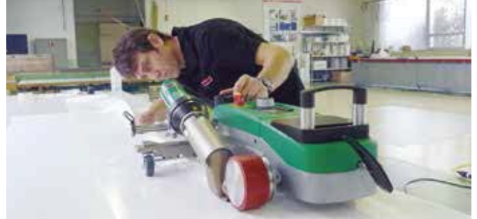
Very easy hem and piping welds with the hem / piping welding kit.
