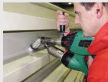
The 45° angled adapter for the WELDPLAST S2 facilitates welding in difficult positions. (accessory)
