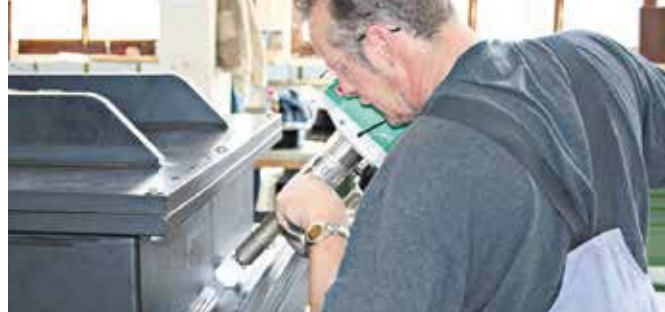
The powerful WELDPLAST S4 in use.
