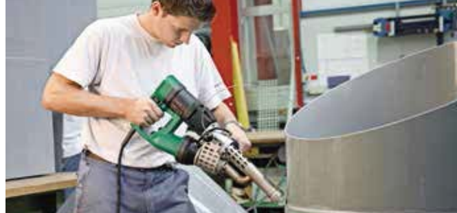
FUSION 3C during the welding of a V-seam.
